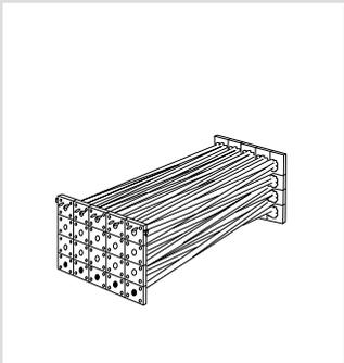
Remove frame from case and place on floor. Stand in front of unit with the yellow dots on bottom and facing you. Grasp upper ends of frame and pull up and outward.
