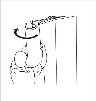
Lift end panel and guide front notch of plastic plate over front peg. Hook the other side on the panel peg at the back of the frame.
