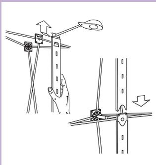
Mount top channel bars (with lights attached) to frame by aligning hole in channel bar over panel pegs on top hub and sliding up. Once top of channel bar is in place, slide channel bar down onto bottom hub to secure.
