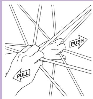
To close the frame, push and pull from the middle of the frame while grasping the hubs as shown. Once the frame starts to collapse, move hands away from the hubs to avoid pinching. Do not pull tubing alone.
