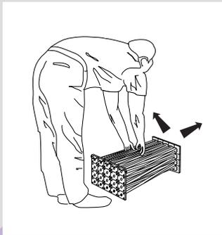
Continue pulling up and outward until the frame is fully expanded. Spacer bars should be close enough to each other to allow for a connection.
