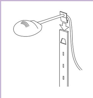
Locate top channel bars. With channel facing away from you, attach lights to top channel bars by inserting light bracket into slot on top of bar.
