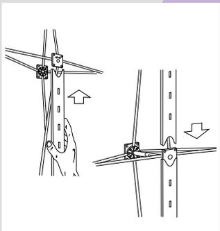
Begin at the bottom center module and attach channel bars by sliding up onto the top hub. Line up the bottom of the channel bar over the lower hub and slide down to secure. Leave the top front row open for top channel bars.
