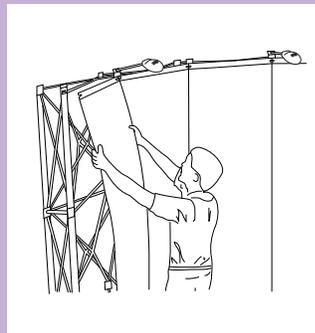
Hold a front panel on its side edges about 1/3 of the way down from the top. Lift section and guide notches over the panel pegs on the top hubs. Slowly release the panel, allowing it to roll down the channel bars. Repeat for all front panels aligning them as you go.
