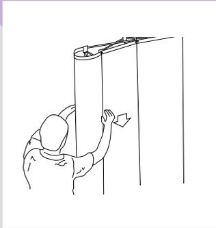
Slowly run your hands down the sides of the panel, attaching magnetic strips to the channel bars and straightening as you go.
